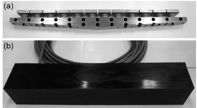
Fig. 1. Photographs of a linear array acoustic transducer with a gradual wedge-shaped tail mass after (b) and before polyurethane molding (a).
